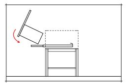
To return the drawer to the unit, fully extend the runners. Tilt the drawer backwards and insert so that the runner intersects the rear of the drawer. Push the runner into the back of the drawer. Locate onto the pins at the front of the runners.
